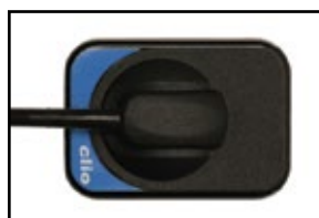
Rounded corners allow for more accurate positioning, especially toward mesial and against palate.
